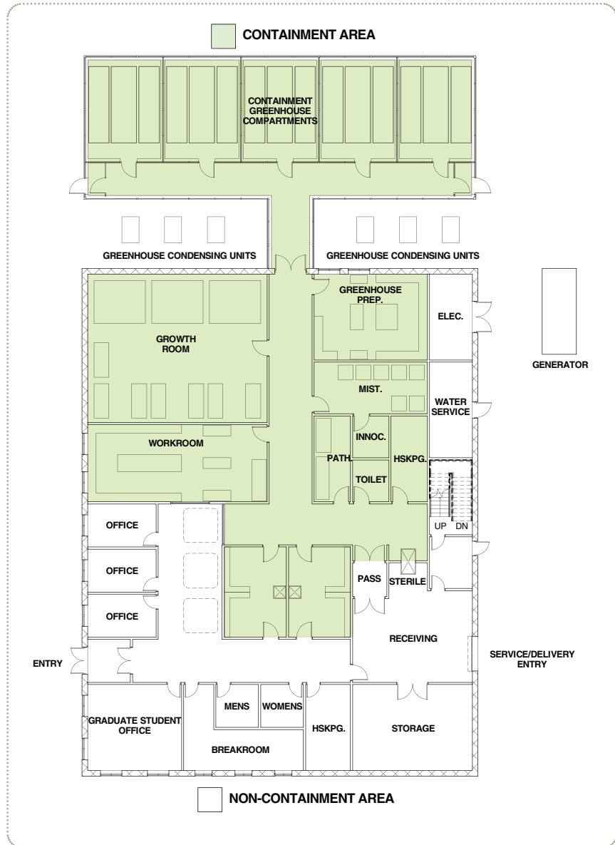
FIGURE 7. Typical Containment Facility Floor Plan*
